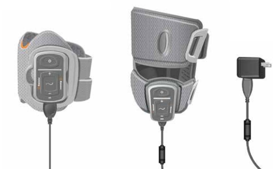
Figure 6-2: L300 Go System Charging Setup (Example of a Lower Leg Cuff and Thigh Cuff Configuration)
