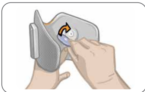
Figure 8-5: Attaching the Cloth Electrodes
