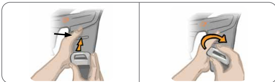
Figure 8-13: Removing the Thigh Straps
